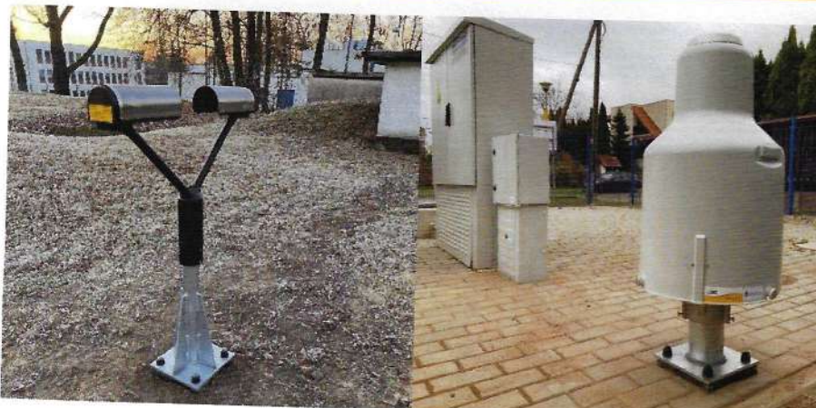
OTT Parsivel Disdrometer (left). OTT Pluvio 2 L and a standing cabinet (right).
