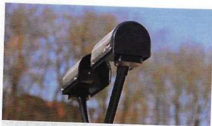
Measuring heads of OTT Parsivel ®
